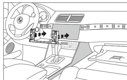
10. Mount the DDIN housing into the radio cavity using the supplied (2) PPH-12 Phillips screws and (2) factory screws removed in disassembly.
