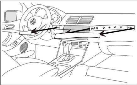
3. Disconnect the wiring. Unclip and remove the wood trim above the glove box and to the left
