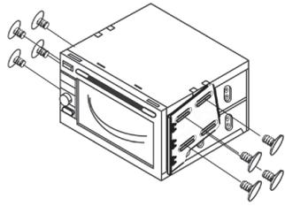
11. Mount the DDIN radio to the supplied DDIN brackets using the supplied (8) ISO screws. Connect all required circuit points. Re-connect negative battery terminal and test the unit for proper operation
