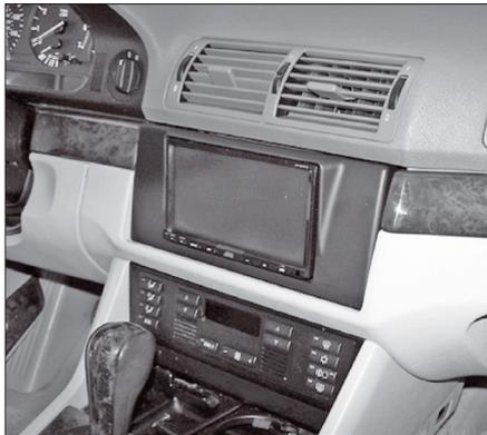
13. Snap the DDIN trim plate over the radio. Reassemble dash in reverse order of disassembly.
