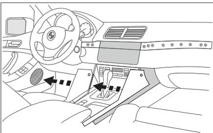
4. Remove the Phillips screws securing the (2) side panels on the center console then slide the panels forward to unclip and remove them.
