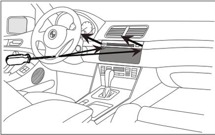
2. Disconnect the wiring. Remove (2) T-10 Torx screws securing the top of the factory radio then unclip and remove.
