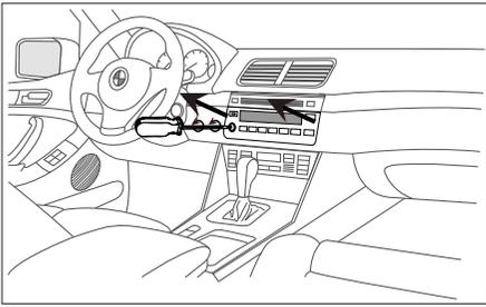
1. Remove the volume by pulling out towards the rear of the vehicle. Using a T-10 Torx screwdriver to turn the release screw 90° behind the volume knob then pull out on the bottom of the radio and remove
