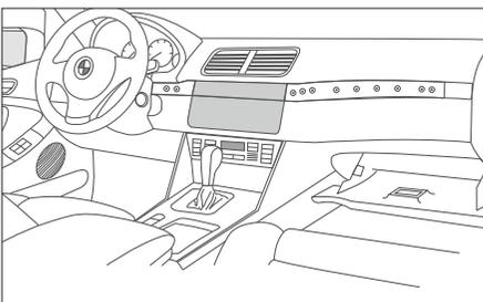
5. Unclip and remove the (2) glove box side supports with the glove box open.
