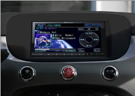
5. Push metal frame into mounting frame. Place both on dashboard
