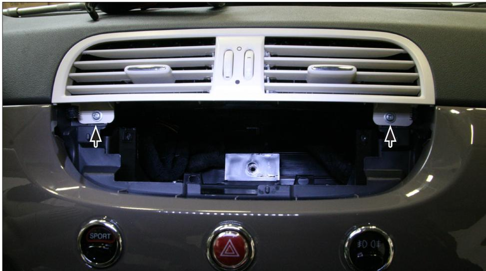
2. Remove 2 screws of air vent cover. Remove air vent cover
