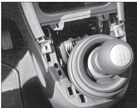
3. Remove the gear lever cap.
