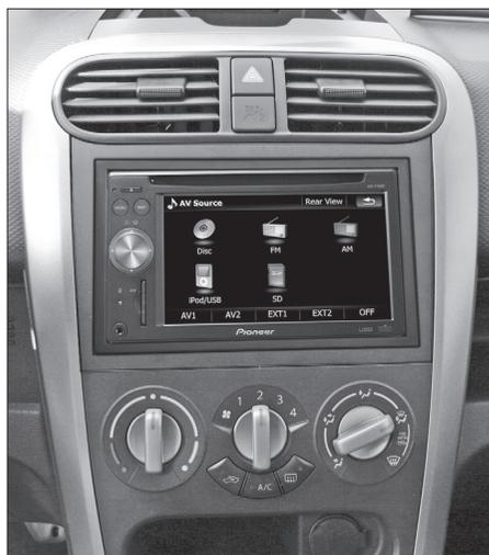
7. Push the Metal Frame into the facia plate, place both into the dashboard.
