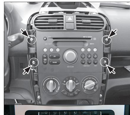
6. Remove the 4 Phillips screws, remove the OEM Radio.
