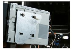
8. Attach mounting frames to double DIN head unit
