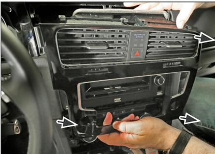
3. Unclip air vents (special VW tool may be required)
