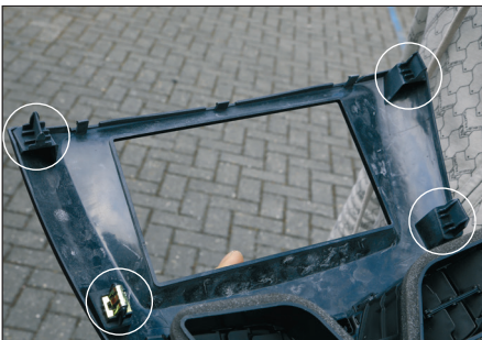
4. Remove 4 clamps from OEM panel Place 4 clamps onto new fascia plate
