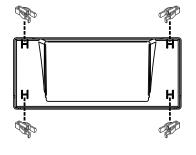
12. Push the included snaps onto the legs of the DDIN Radio trim plate.
