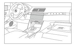
7. Remove the Phillips screws securing the glove box to the lower dash panel and let it hang.
