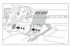
Remove the Phillips screws securing the (2) side panels on the center console then slide the panels forward to unclip and remove them.
