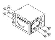
11. Mount the DDIN radio to the supplied DDIN brackets using the supplied (8) ISO screws. Connect all required circuit points. Re-connect negative battery terminal and test the unit for proper operation
