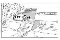
10. Mount the DDIN housing into the radio cavity using the supplied (2) PPH-12 Phillips screws and (2) factory screws removed in disassembly.
