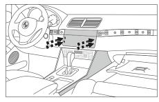
9. Remove the (4) Phillips screws securing the radio sub dash panel to the lower dash panel. Pull the right side of the lower dash panel outward to gain access to and remove the radio sub dash panel.
