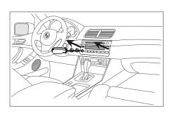
1. Remove the volume by pulling out towards the rear of the vehicle. Using a T-10 Torx screwdriver to turn the release screw 90° behind the volume knob then pull out on the bottom of the radio and remove
