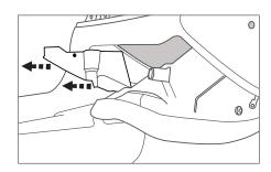
6. Remove (2) Phillips screws securing the panel on the inside left hand side of the glove box then remove the panel.
