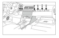
8. Remove the Phillips screws above the glove box and the one behind the cover on the side of the lower dash panel. Remove the two screws on the lower dash panel to the left of the radio.
