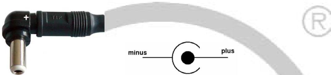
If the marking (+) and the signature TIP are readable, rests against the plug exterior minus and the plug inside plus.
