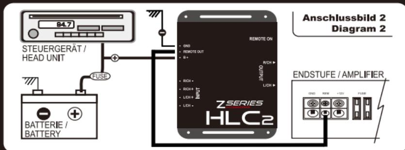
First disconnect the power supply (battery) of the vehicle. Connect the **speaker output** from the head unit (radio) to the „High Level“ INPUT of the HLC<sub>2</sub>. Pay attention for the right way of connection.
