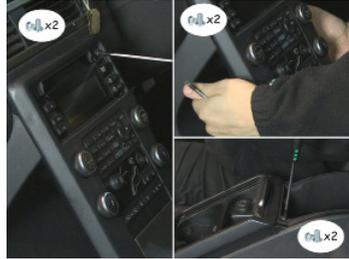
3. Pull the trim surrounding the gear stick up to reveal **another** 4 screws that will need to be removed.
