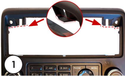
**1.** Cut bottom of clips where **highlighted**.
