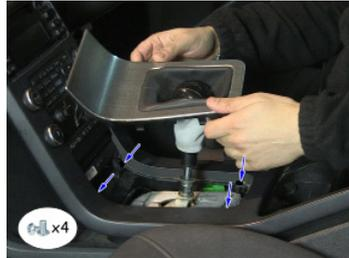
4. Once all of the following screws have been removed, take hold of the main panel and firmly pull it away from the dashboard.
