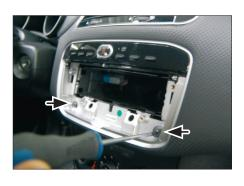
1. Remove OEM head unit with radio release keys
