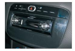
Remove 4 screws.Remove Switch panel from the OEM trim frame
