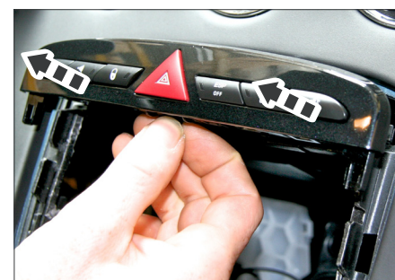
7. Remove top panel Remove buttons
