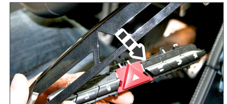
7. Remove top panel Remove buttons
