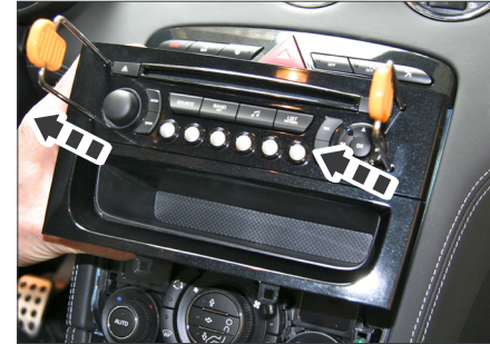
5. Remove OEM head unit
