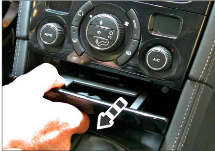
1. Remove lower tray under OEM head unit
